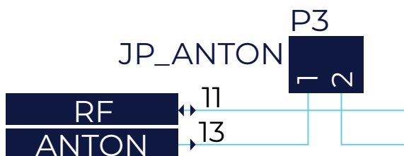
Figure 6 – Jumper to connect or disconnect the power to the GPS external antenna
